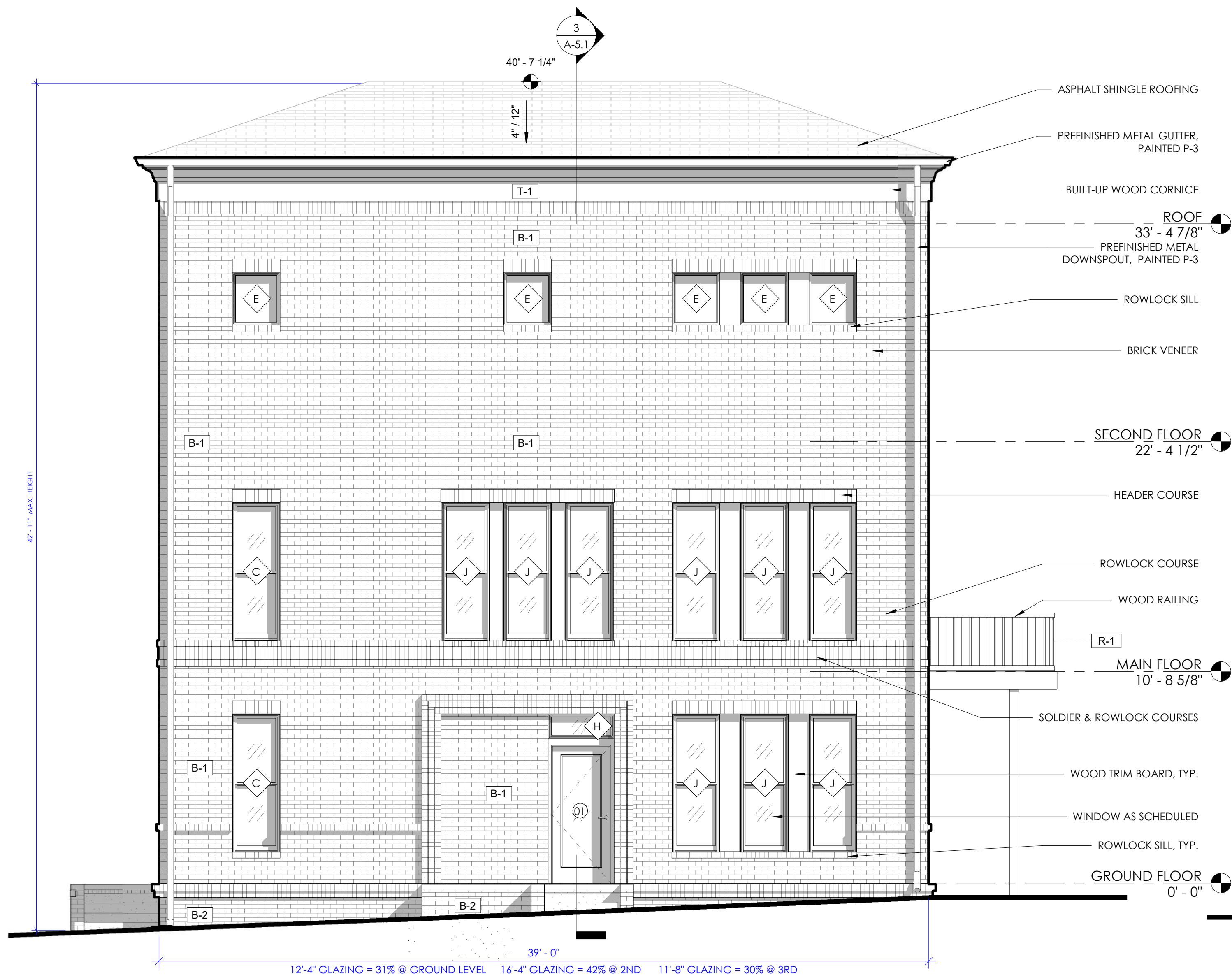
2 1/4" = 1'-0" BUILDING 1 - EAST ELEVATION
