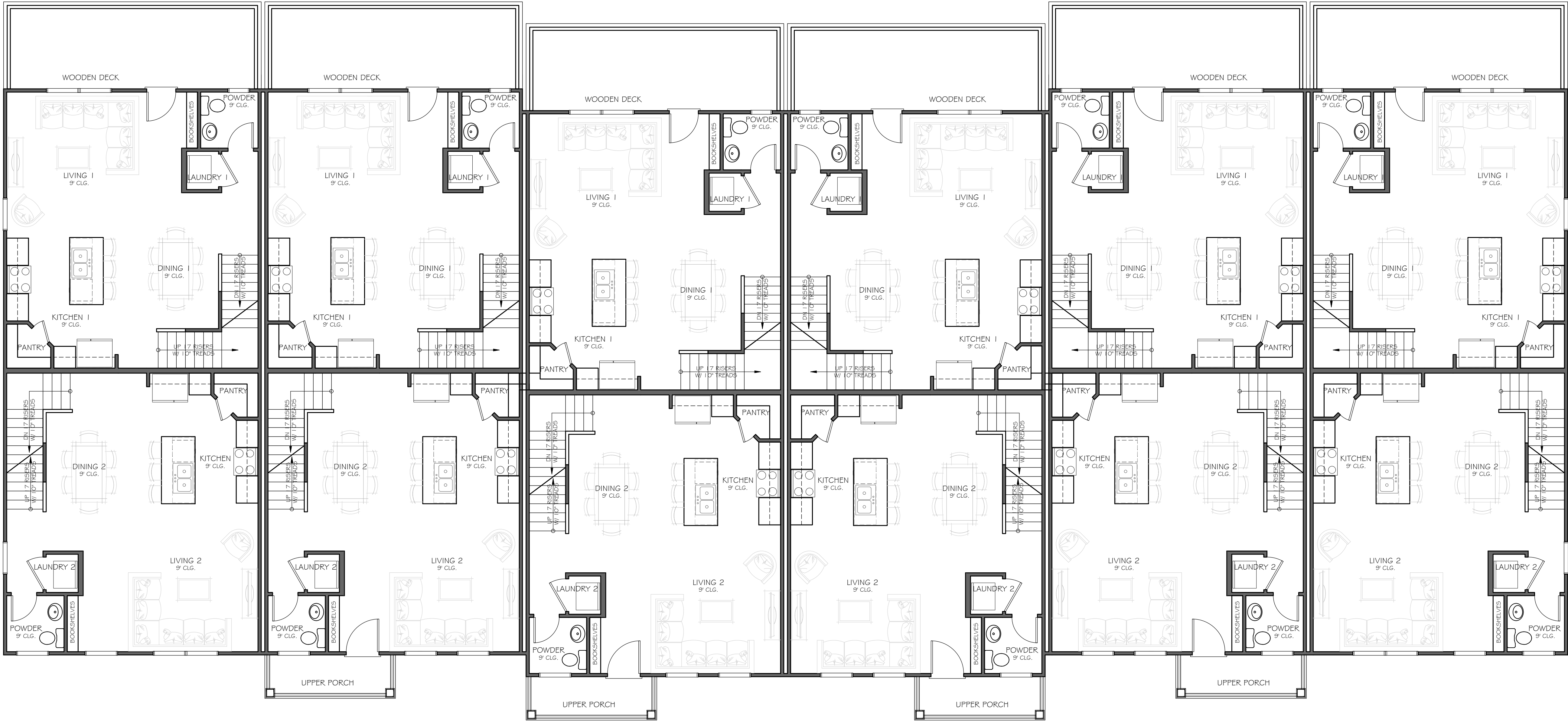
1 1ST. FLOOR (12 UNIT 24x52 PLAN) SCALE: 3/16" = 1'-0"
