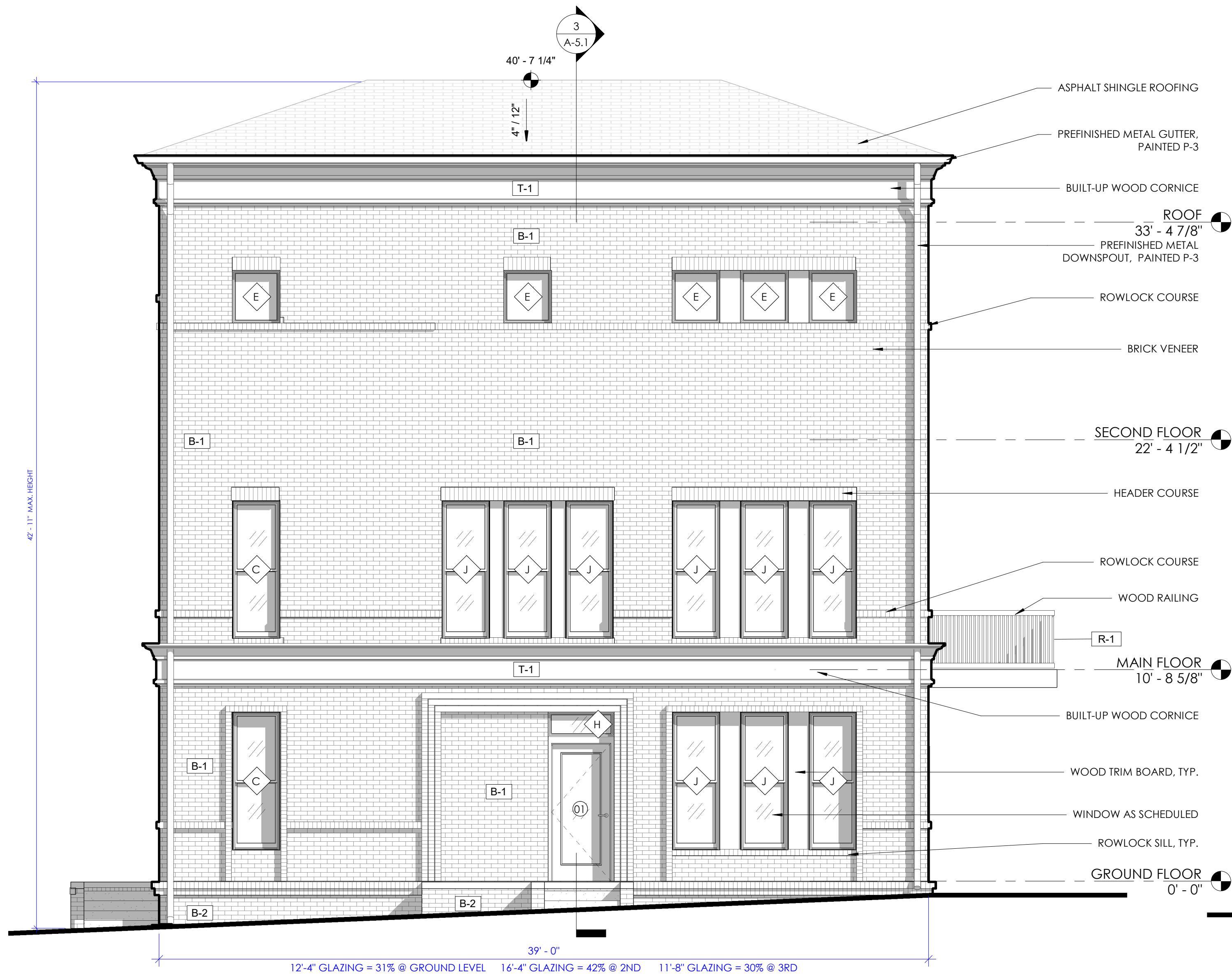
2 1/4" = 1'-0" BUILDING 1 - EAST ELEVATION
