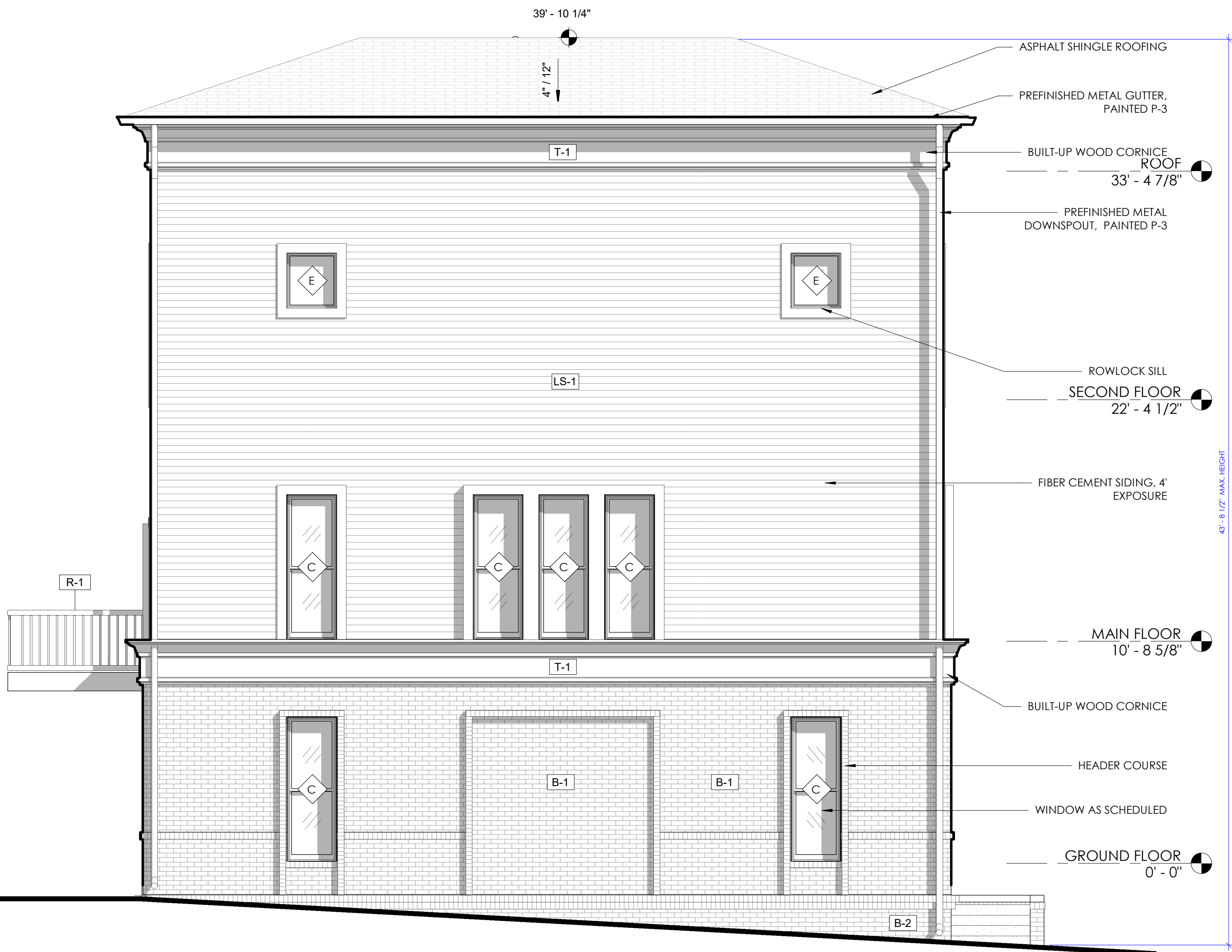
1 1/4" = 1'-0" BUILDING 1 - WEST ELEVATION
