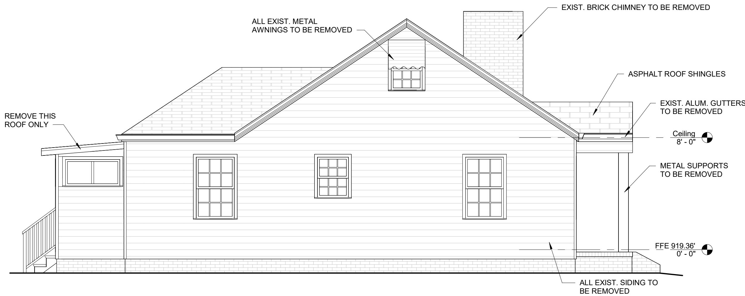
③ EXISTING WEST SIDE ELEVATION 1/4" = 1'-0"
