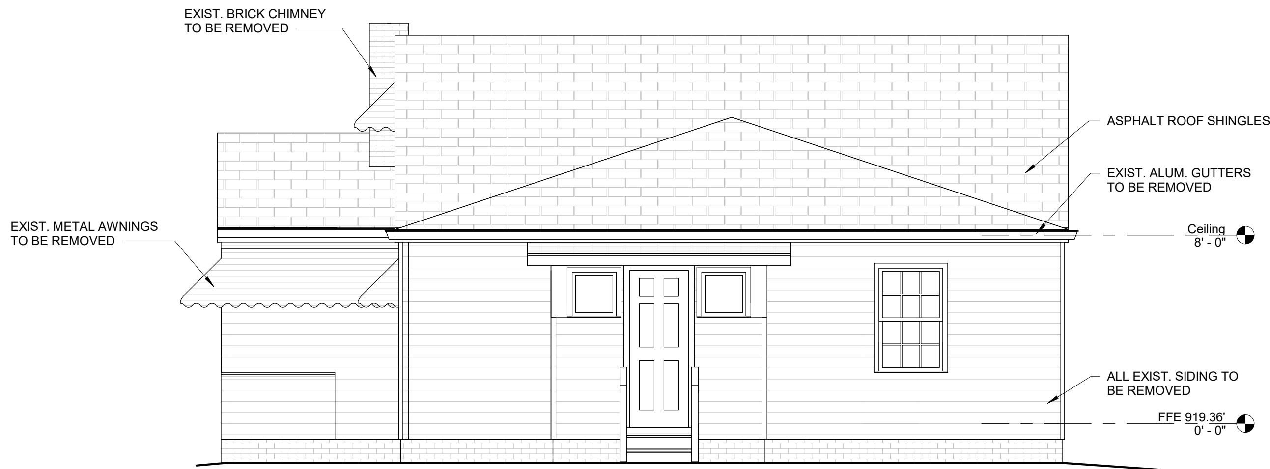
① EXISTING BACK ELEVATION 1/4" = 1'-0"
