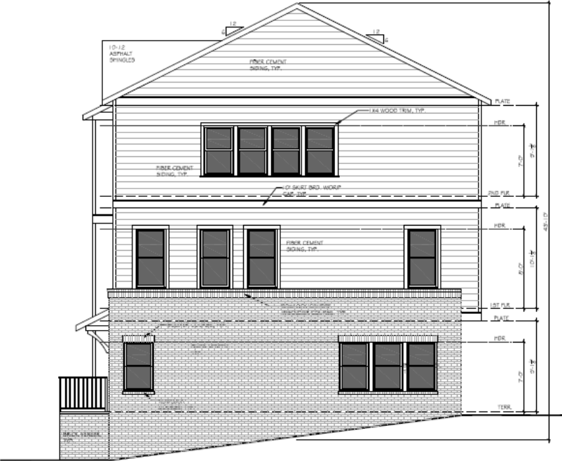
1 RIGHT ELEVATION (BLDG. 1000) SCALE: 3/16" = 1'-0"
