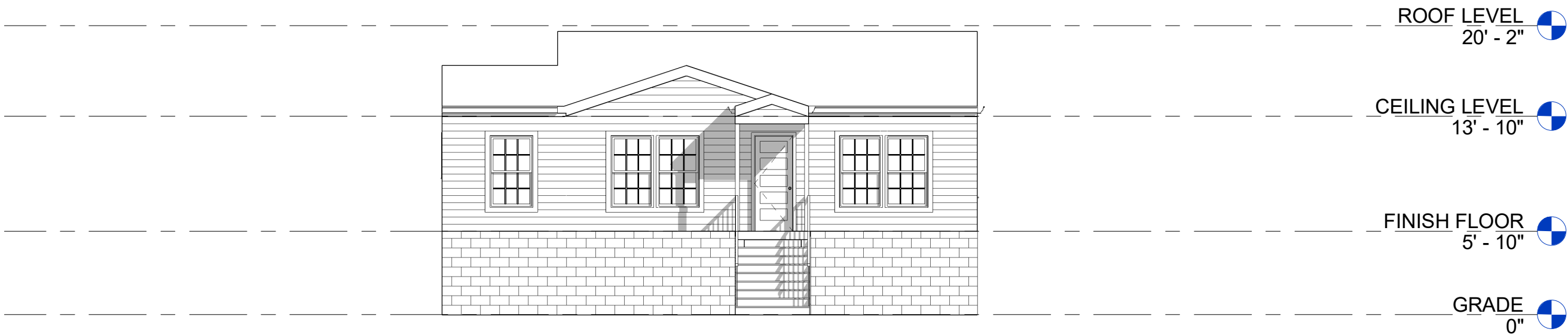
2 EXISTING FRONT ELEVATION 1/8" = 1'-0"
