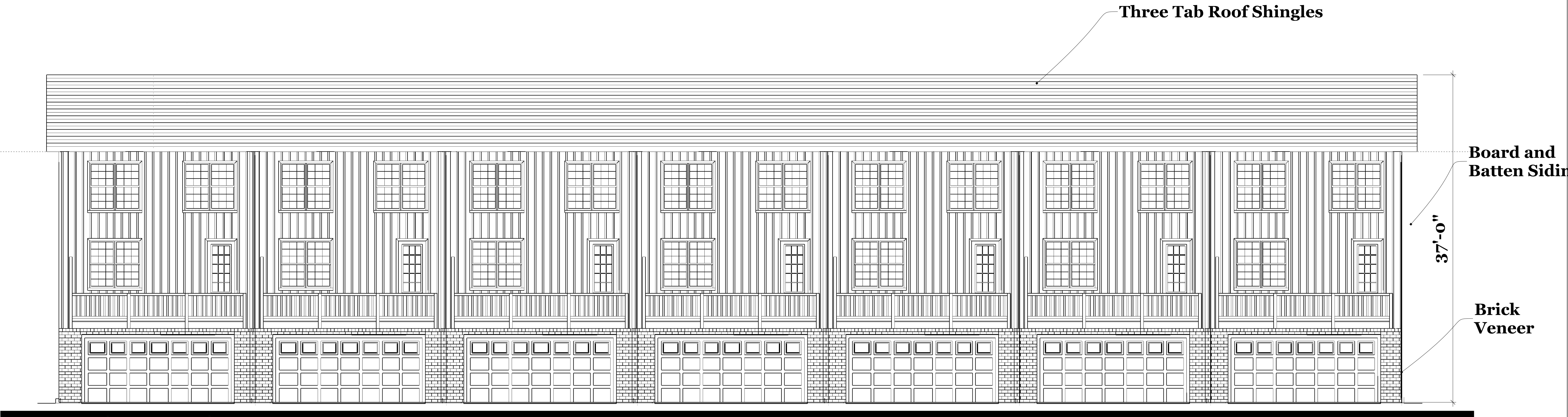
Front Side Typical Building Elevation 3/16" = 1'-0"
