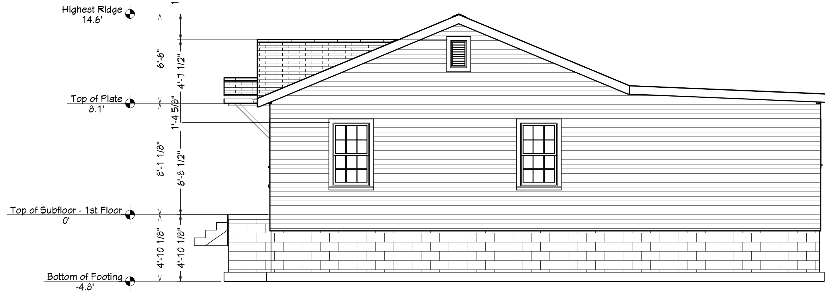
Existing Elevation Right Scale: 1/4" = 1'
