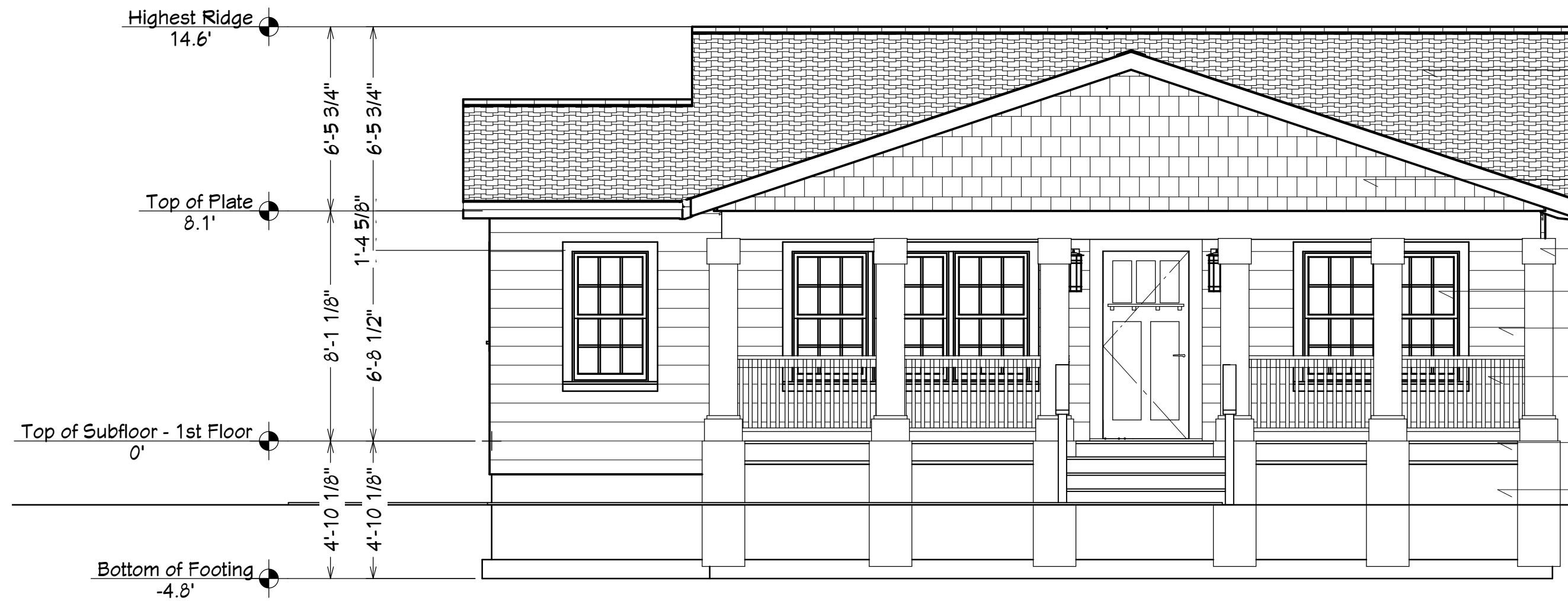
Proposed Elevation Front Scale: 1/4" = 1'
