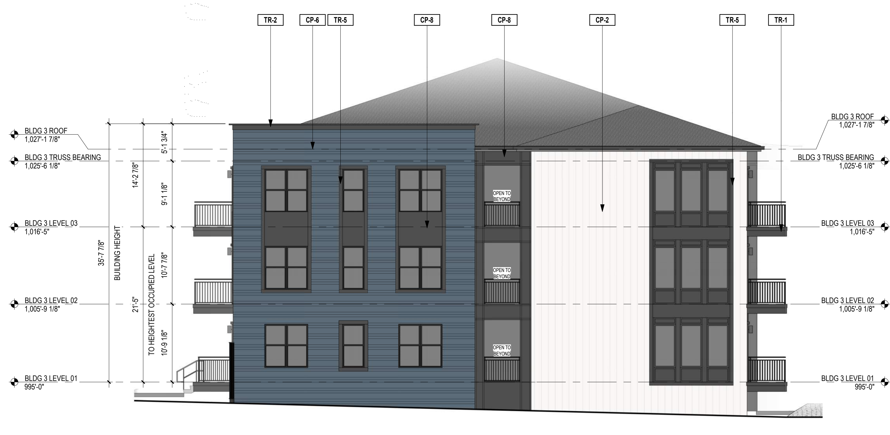
1 BLDG TYPE A - 300 - SOUTH WEST ELEVATION
