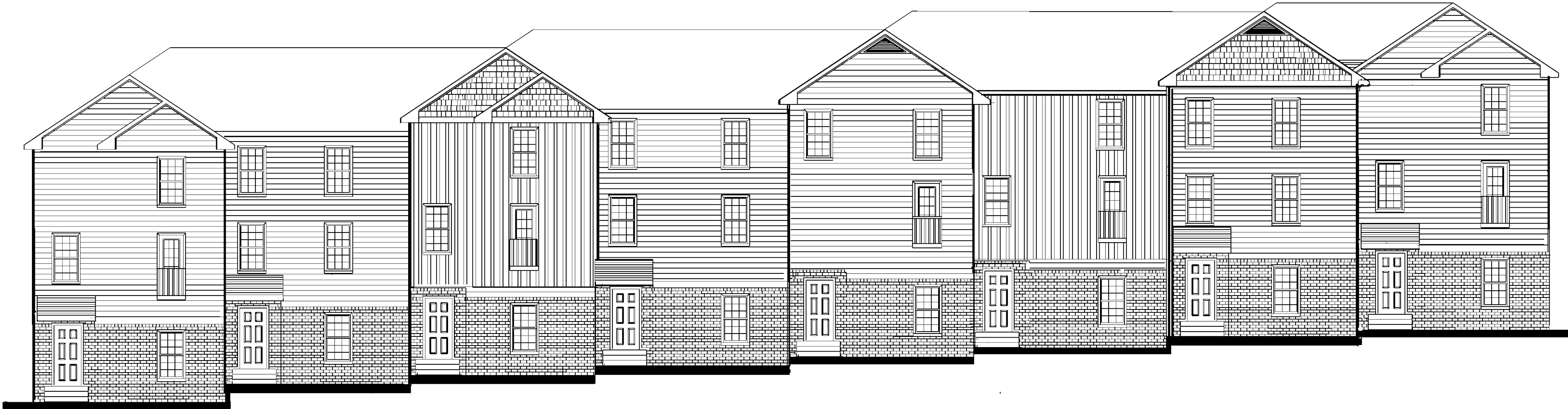
8 Unit Stepped Building Front Elevation 1/8" = 1'-0"
