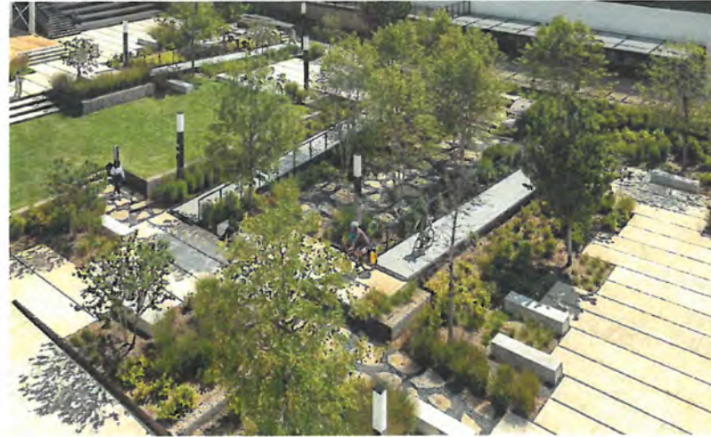
REPURPOSED CHUNKS OF EXISTING CONCRETE IN PEA GRAVEL
