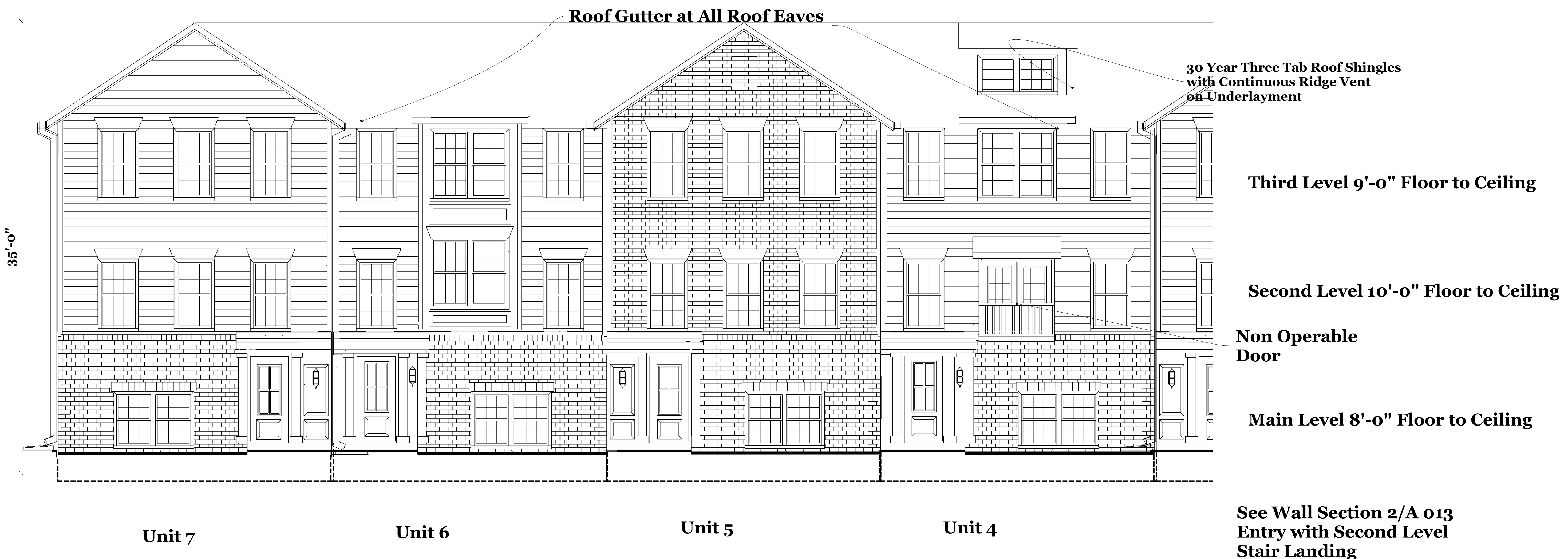
Seven Unit Building Front Elevation 1/4" = 1'-0"
